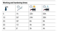
Minimum resin temperature for injection: +10  $^{\circ}\text{C}$  Minimum concrete temperature for injection: +5  $^{\circ}\text{C}$
