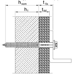
Intended use SDF-10H in a weather shell (hnom)
