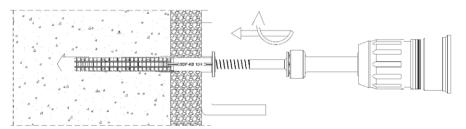
4. Correctly installed anchor
