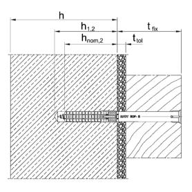
Intended use SDF-10V in solid block (h<sub>nom2</sub>) screw head-type: countersunk (S)
