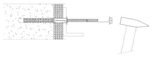
3. Screw in the screw until the head is rested on the plastic sleeve
