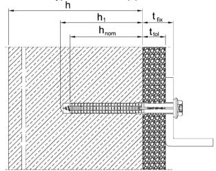
Intended use SDF-10H in concrete/masonry/ autoclaved aerated concrete (h<sub>nom</sub>) Screw head-type: collar head (KB)
